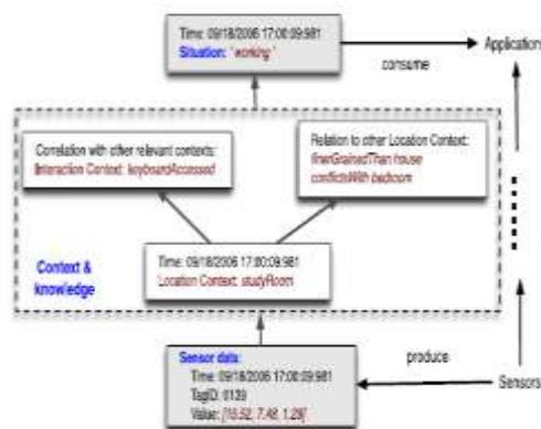
**Fig. 1. Information flow in pervasive computing.**
